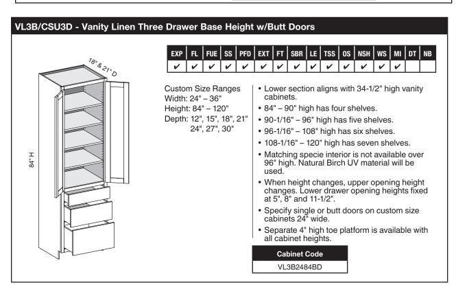
Options Key: EXP = Exposed End(s) FL = Flush End(s) FUE = Flush Unexposed End(s) SS = Shaped Side PFD = Prep for False Door
