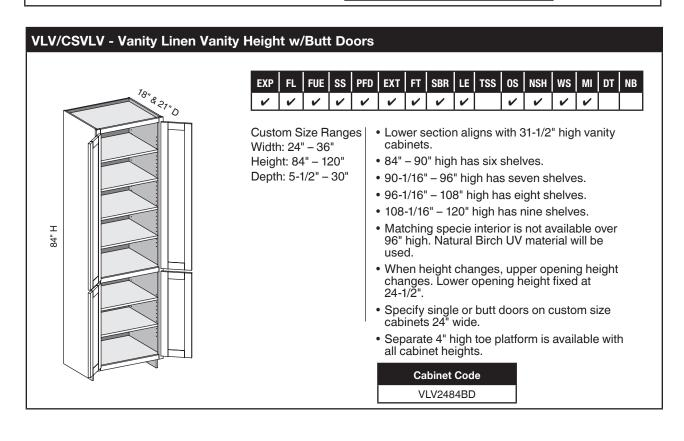
Options Key: EXP = Exposed End(s) FL = Flush End(s) FUE = Flush Unexposed End(s) SS = Shaped Side PFD = Prep for False Door EXT = Extended Stile(s) FT = Flush Toe SBR = Shaped Bottom Rail LE = Leg Extension TSS = Toe Space Side OS = Omit Shelving
