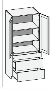
Custom Size Ranges Single Door Width: 12" – 24" Butt Door Width: 24" – 36" Height: 84" – 96" Depth: 12", 13", 15", 16", 18", 21", 24", 27", 30"
