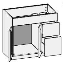
Custom Size Ranges Single Door Width: 30" – 36" Butt Door Width: 36" – 48" Height: 31-1/2" – 34-1/2" Depth: 12", 13", 15", 16", 18", 21", 24", 27",
