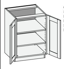
Custom Size Ranges Single Door Width: 9" – 24" Butt Door Width: 24" – 36" Height: 10" – 42" Single Door Depth: 12" – 30" Butt Door Depth: 12" – 30"
